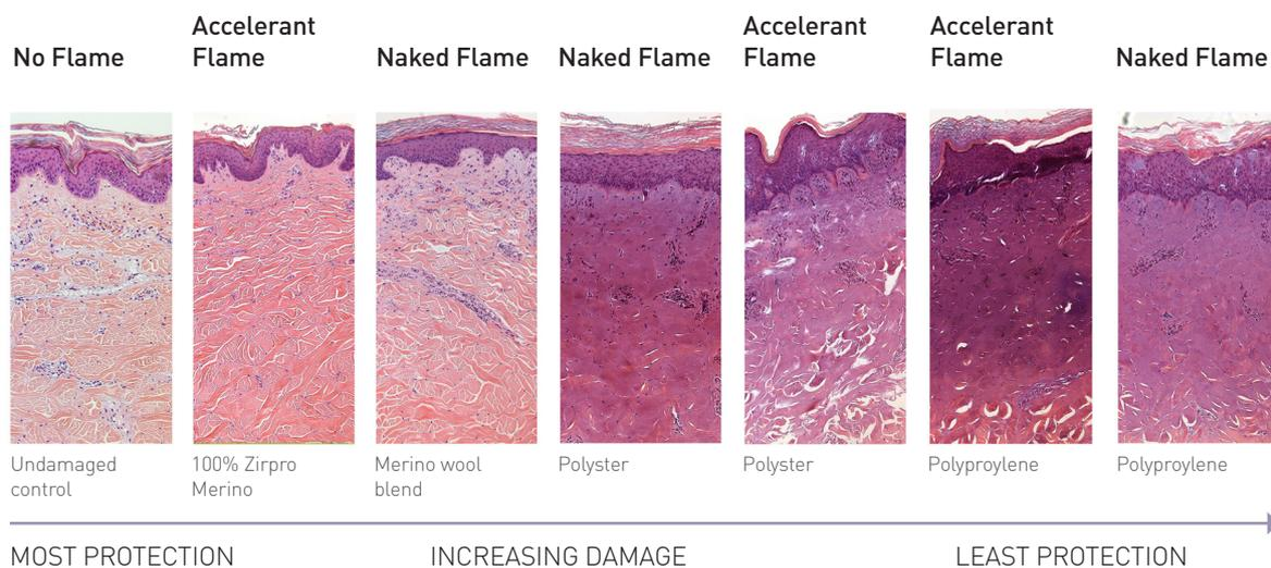
Figure 1: Simulated exposure to naked flame ignition and accelerant fuelled threat
